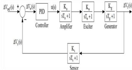
Fig. 2. AVR Diagram Block with PID [2].
