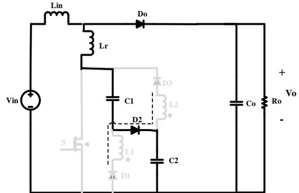
Fig. 7. The equivalent circuit operation of the proposed converter in the fifth Mode.
