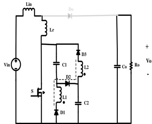
Fig. 4. The equivalent circuit operation of the proposed converter in the second Mode.
