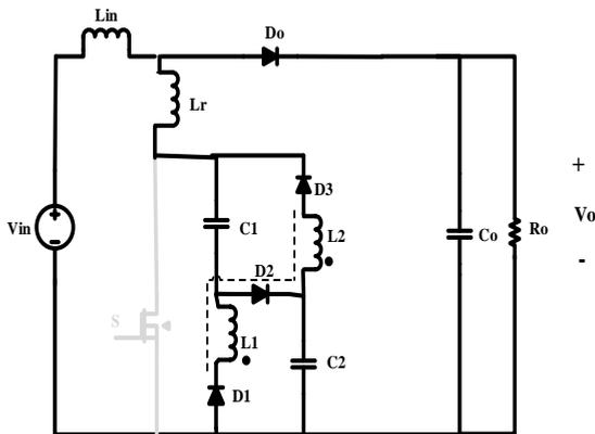
Fig. 6. The equivalent circuit operation of the proposed converter in the fourth Mode
