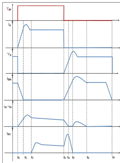
Fig. 2. Key waveforms of the proposed Boost converter with lossless snubber.
