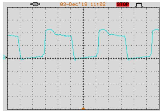
Fig. 15. Current waveform of  $D_0$  in the Proposed Boost Converter (2 A / div), Time (2.5μs / div).
