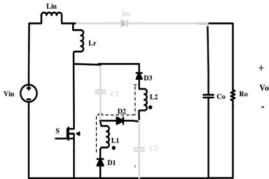
Fig. 5. The equivalent circuit operation of the proposed converter in the third Mode.
