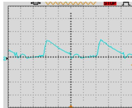
Fig. 14. Current waveform of  $D_3$  in the proposed boost converter (1 A / div), time (2.5μs / div).
