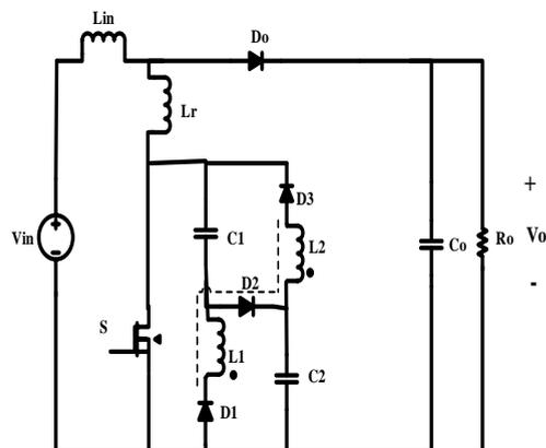
Fig. 1. The introduced boost converter with proposed snubber circuit.
