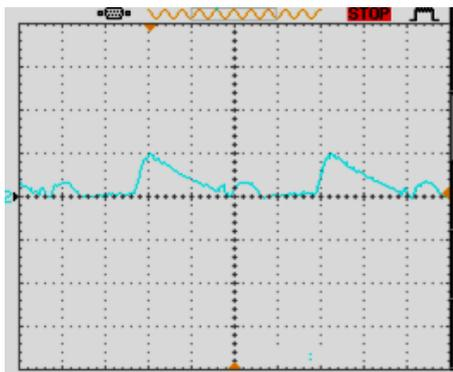
Fig. 12. Current waveform of  $D_1$  in the proposed boost converter (1A / div), time (2.5μs / div).
