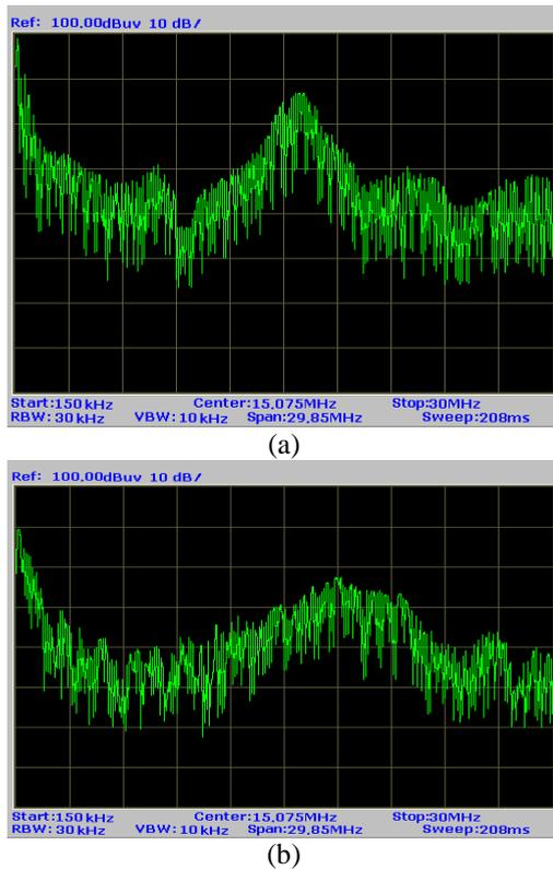
**Fig. 18.** Measured EMI Conductivity (a) Hard Switching Boost Converter, (b) Proposed Boost Converter (Vertical axis: 20–100 dBμV, horizontal axis: 0.15–30 MHz).
