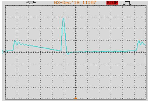
Fig. 13. Current waveform of  $D_2$  in proposed boost converter (1A / div), time (1μs / div).
