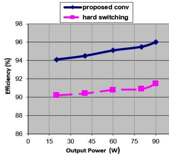
**Fig. 19.** The proposed Boost Converter efficiency compared to its hard switching counterpart.
