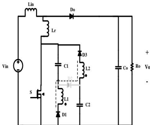
Fig. 3. The equivalent circuit operation of the proposed converter in the first Mode.
