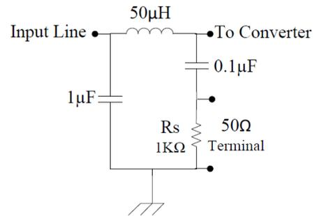
Fig. 17. CISPR22 LISN Model for Measurement of Conductive Electromagnetic Interactions [17].
