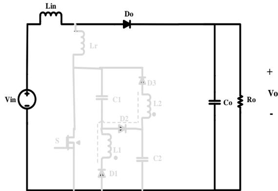
Fig. 9. The equivalent circuit operation of the proposed converter in the seventh Mode.
