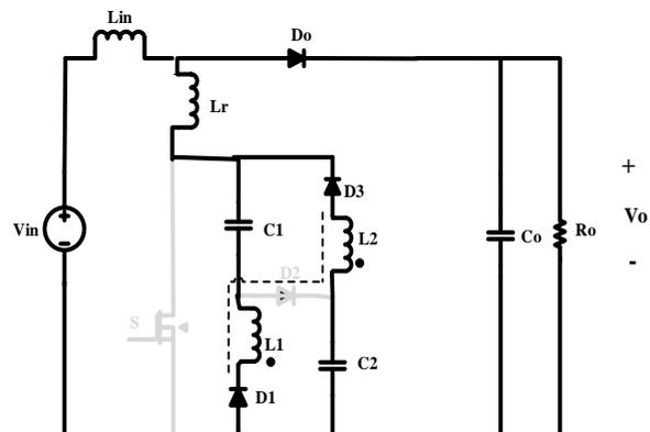
Fig. 8. The equivalent circuit operation of the proposed converter in the sixth Mode
