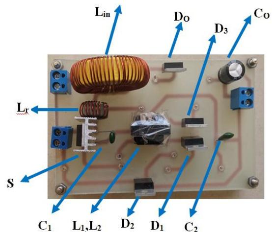
Fig. 10. Proposed Boost Converter Circuit.
