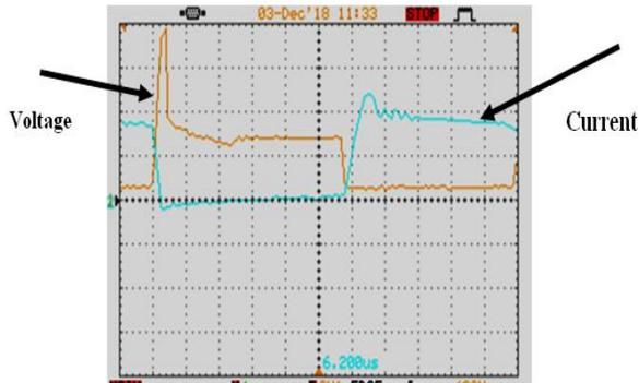
Fig. 11. The voltage and current waveforms of the switch (50V / div, 2A / div, 1μ s / div).
