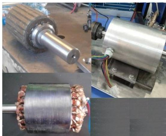
**Fig. 11.** Rotor core, Stator core with windings and prototyped machine.
