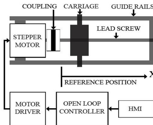
**Fig. 4.** The schematic model of the mechatronic part.
