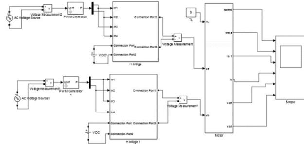
Fig. 7. The overall design of the simulation.
