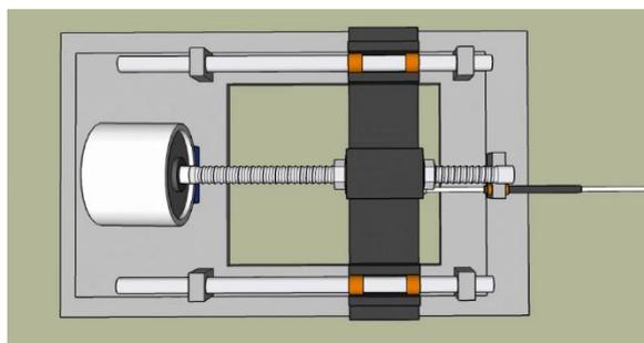
**Fig. 3.** The 3D model of the designed translation system.
