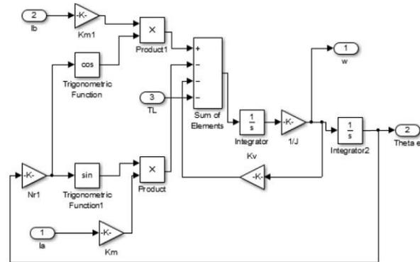
Fig. 8. Speed and Position subsystems.
