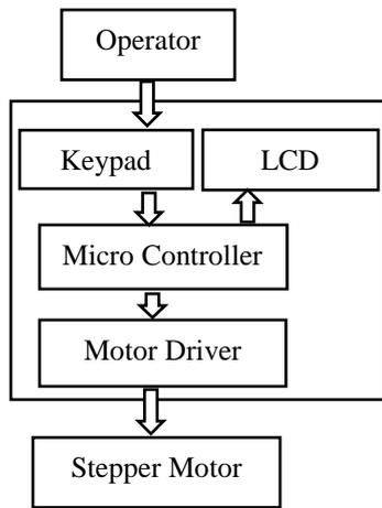
Fig. 5. The block diagram of the controller.
