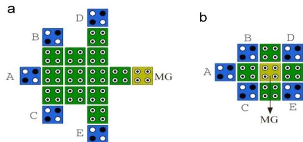
Fig. 3. Majority Gate of 5 inputs: (a) introduced sample in [16], (b) introduced sample in [15].
