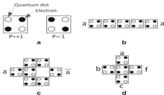
**Fig. 1.** Elements in QCA: (a) QCA cell, (b) binary wire, (c) inverter, (d) majority gate of three inputs base.
