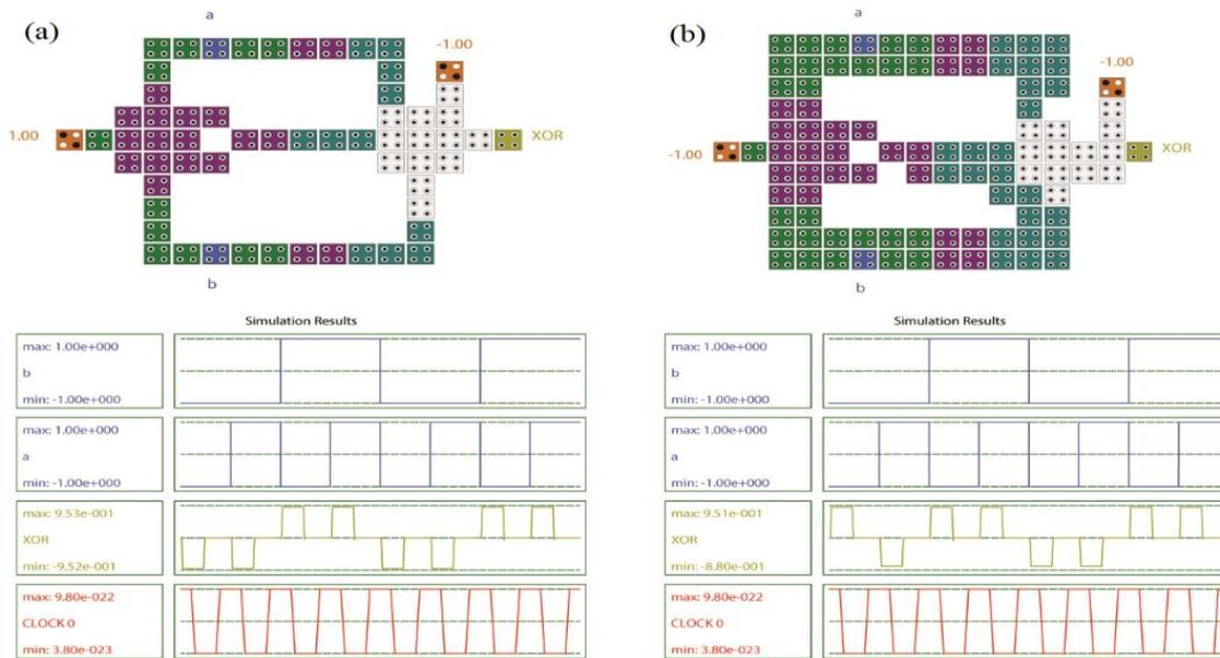
**Fig. 7.** The structure and form of the introduced new wave of the gates: (a) structure and waveform of the first fault tolerance of XOR gate that are used in this gate with tile structure in majority gates, (b) Structure and Waveform XOR second fault tolerant which is also used in tile structures in addition to majority gates in the wiring.
