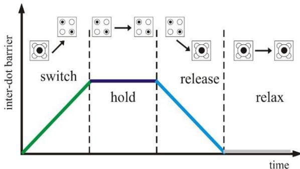
Fig. 2. QCA Clocking Mechanism in four phases.
