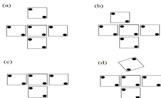
Fig. 5. Some common defects in QCA: (a) cell displacement, (b) cell misalignment defects, (c) missing cell, (d) cell rotation.
