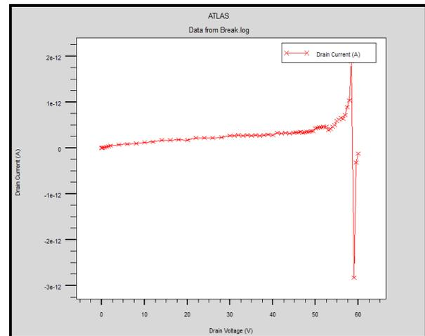
Fig. 4. Drain current versus drain voltage for  $V_g=0$ , in order to obtain breakdown voltage.
