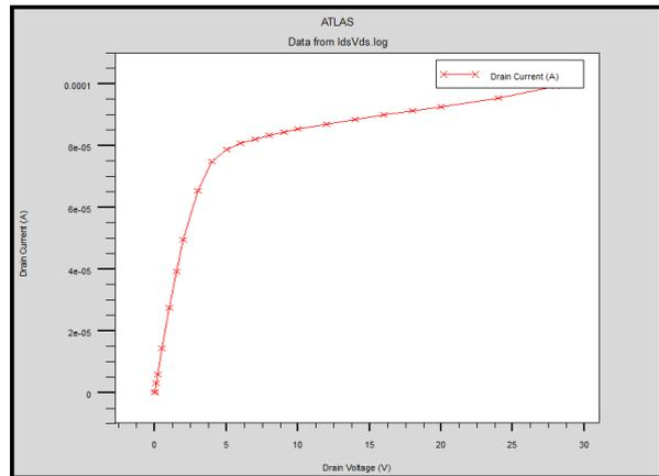
Fig. 7. Drain current versus drain voltage.
