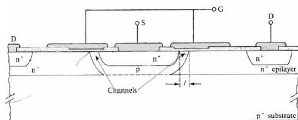
Fig.1. Cross section view of LDMOS transistor.
