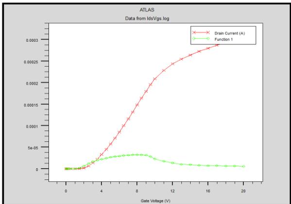
Fig. 6. Current changes diagram in terms of gate voltage changes in order to obtain transconductance.
