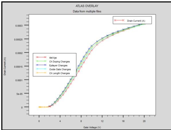
Fig. 8-a. The results of changes in threshold voltage.
