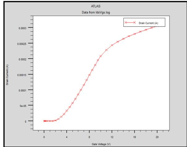
Fig. 3. Drain current versus gate voltage in order to obtain the threshold voltage.
