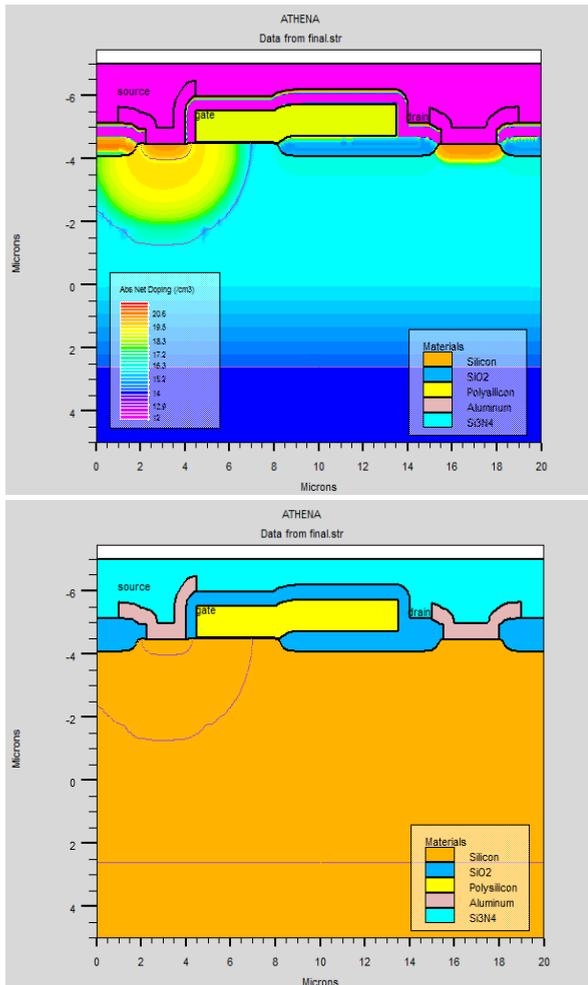
Fig.2. The structure of LDMOS transistor.
