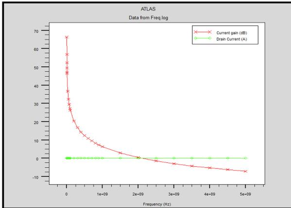
Fig. 5. Current gain diagram in terms of frequency in order to obtain cut-off frequency.
