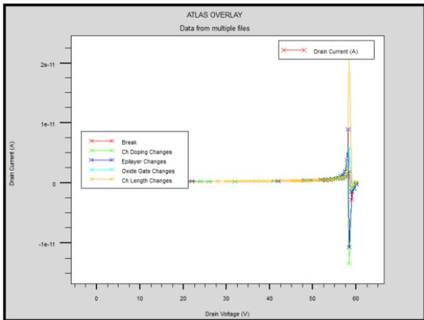
Fig. 8-b. The results of changes in breakdown voltage.
