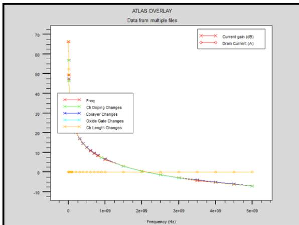
Fig. 8-c. The results of changes in cut-off frequency.
