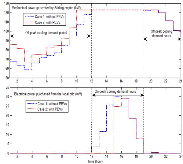
Fig. 8. Mechanical power generated by Stirling engine and electrical power purchased from the upstream grid.
