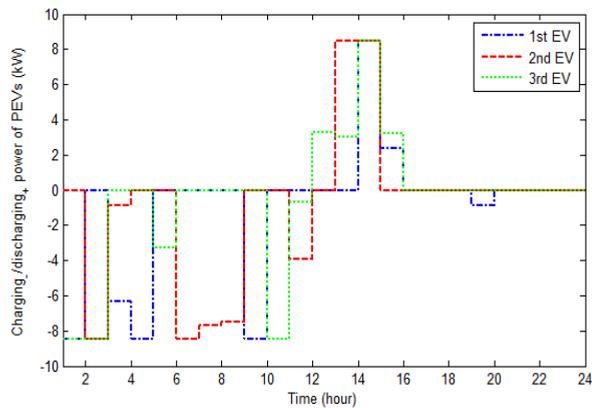
Fig. 7. Charging and discharging patterns of PEVs.
