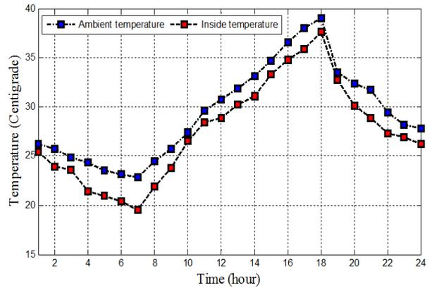
Fig. 5. Ambient and indoor air temperatures during a sample summer day before installing the cogeneration system
