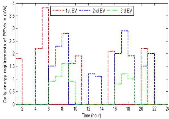
Fig. 6. Daily driving patterns of three different PEVs.
