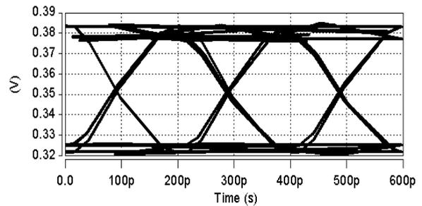
Fig. 6. Simulated Eye-Diagram of the Proposed TIA for 100 $\mu$ A 5Gbps NRZ PRBS7
