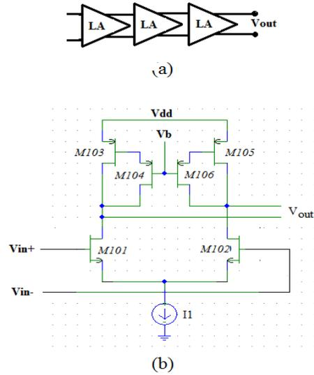
Fig. 13. (a) Block diagram of the Limiting Amplifier (b) Structure of each cell gain
