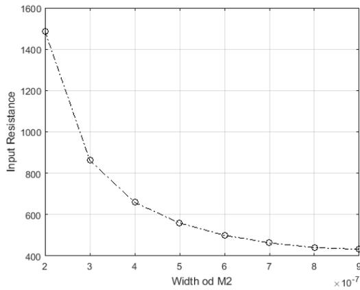
Fig. 8. Width of M2 vs. input resistance
