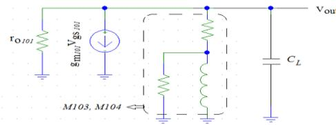
Fig. 14. Equivalent circuit of each cell gain of LA stage
