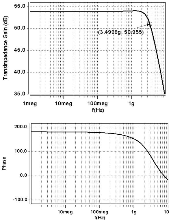
Fig. 4. (a) Frequency response (b) Phase of the proposed TIA.
