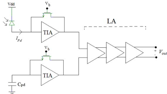
Fig. 15. Block diagram of the proposed optical receiver
