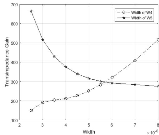
Fig. 10. Width of M5 and M4 vs. gain
