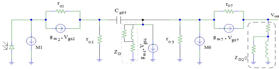
Fig.3. Small signal equivalent circuit of the proposed TIA
