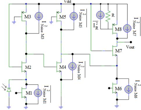
Fig. 11. Equivalent noise circuit
