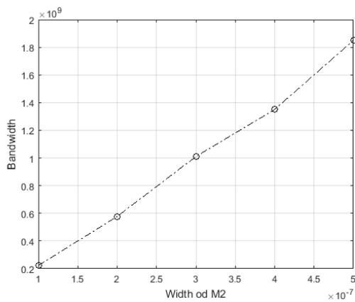
Fig. 9. Width of M2 vs. bandwidth
