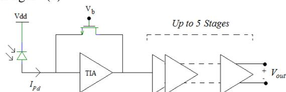
**Fig. 1.** Block diagram of a typical optical communication receiver
