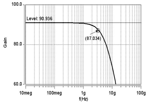
Fig. 16. Frequency response of the optical receiver system
