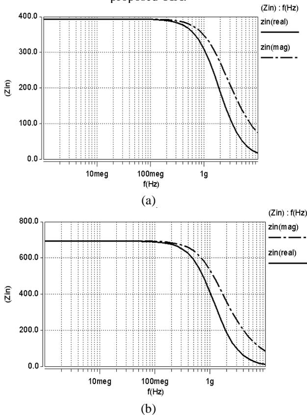
Fig. 5. Input impedance and input resistance (a) with feedback (b) without feedback network.
