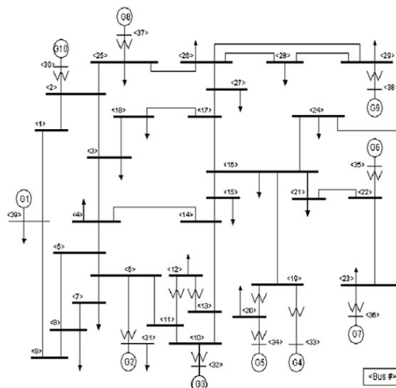
Fig. 3. IEEE 39 bus single line diagram.
