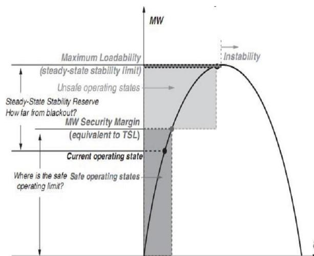
Fig. 1. Secure and Insecure operation states.
