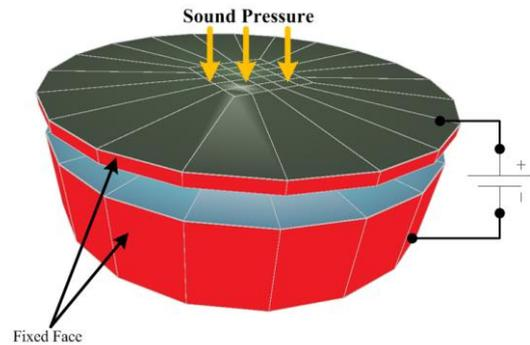
Fig. 4. Simulation setup for flat sensor.
