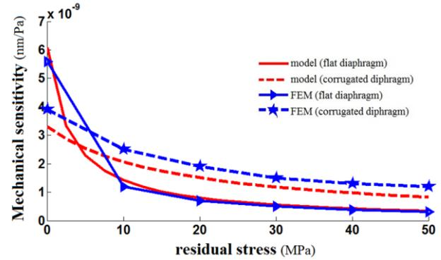
**Fig. 7.** Mechanical sensitivity of corrugated and flat diaphragm.
