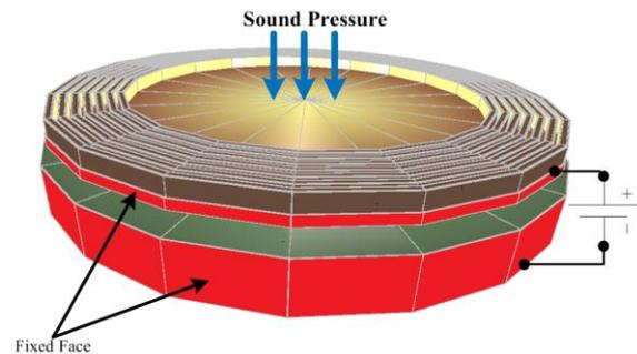
Fig. 5. Simulation setup for corrugated sensor.
