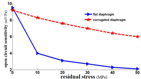
**Fig. 9.** Open-circuit sensitivity of acoustic sensor.
