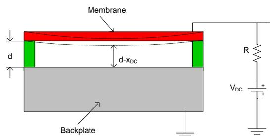
**Fig. 1.** Schematic of condenser acoustic sensor.
